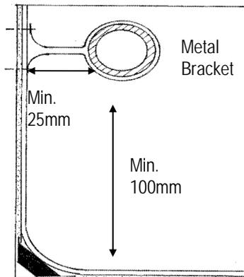
Figure 3a Service Pipe Clearance
