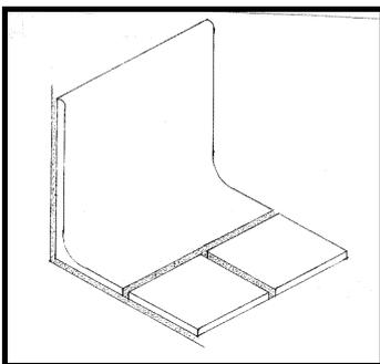
**Pre-formed tiles** without any hollow formed behind and grouted as required for the floor surface. (Figures 1a & 1b)
