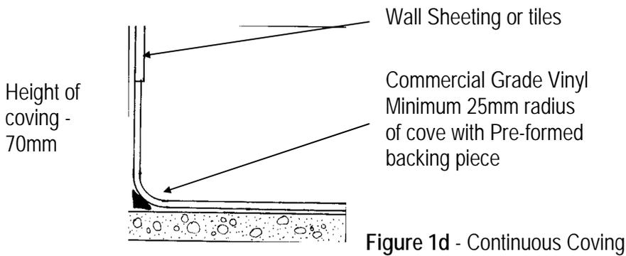
**Continuation of the floor surface material** up the wall, adequately supported with a pre-formed backing piece if not integral with the floor base. (Figure 1d)
