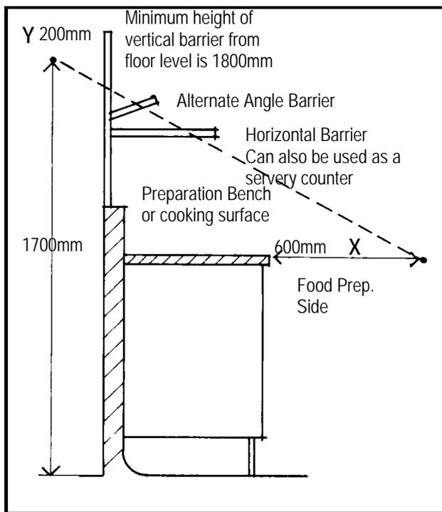
Where "X" is a point measured 600mm horizontally from the preparation bench or cooking surface.
