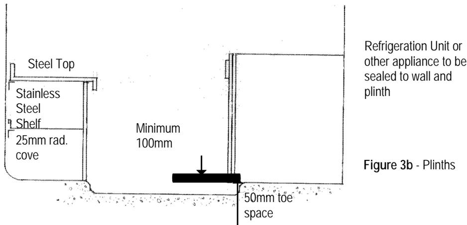
In wet areas benches, table tops, shelving and brackets etc should be constructed of stainless steel. Storage shelving should be kept 25mm clear of walls and vertical surfaces to eliminate any dirt or other material gathering at the rear of shelving in hard to reach places.
